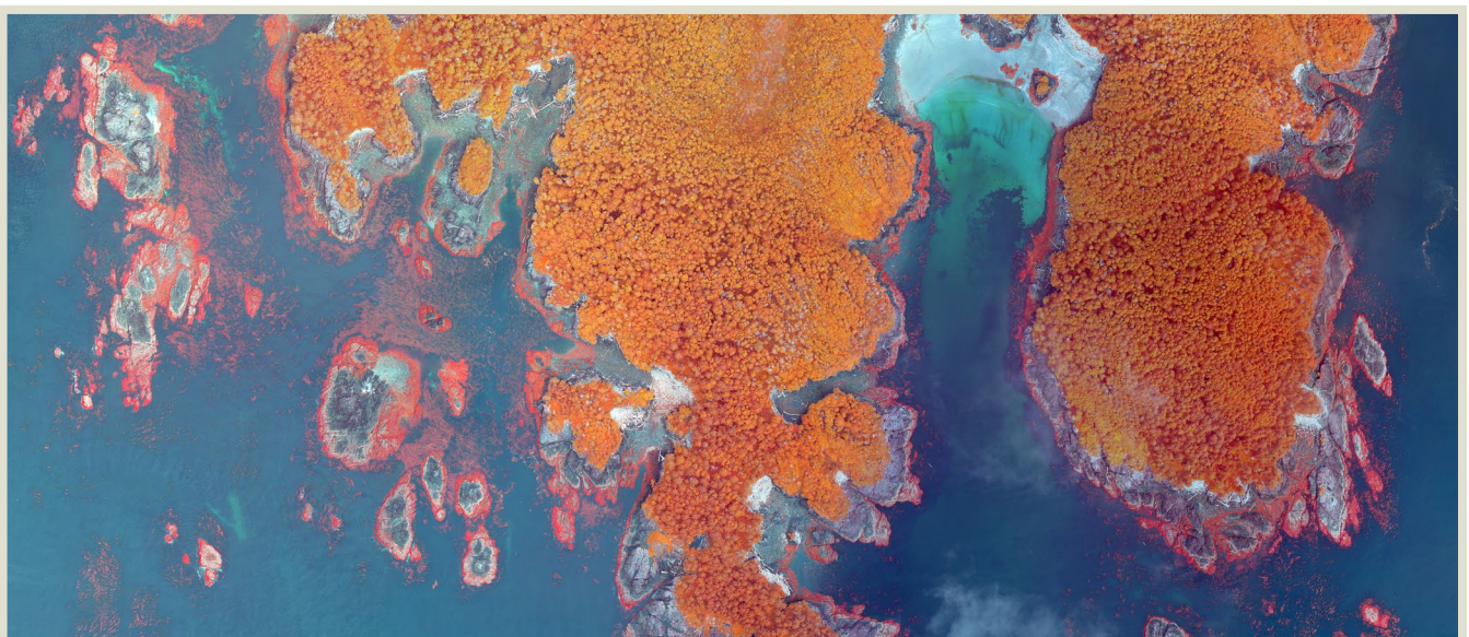
4-band imagery acquired from Phase-1 cameras mounted on a fixed-wing aircraft. Image shown in false-color NIR. Image: Hakai Institute.
